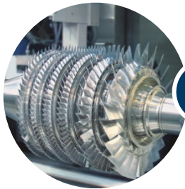
1 High-pressure compressor (HPC)
